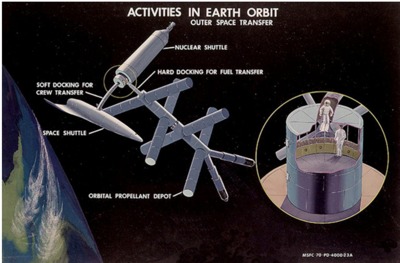
An early concept drawing for an orbiting propellant depot servicing a nuclear shuttle. Image: NASA
