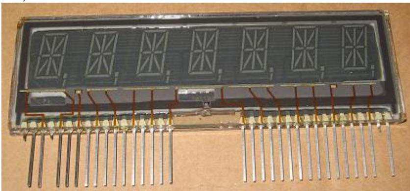
Install the glass into the board as normal but insert Pin #0 into Hole #1 and Pin #2 into hole #2... etc all the way down the line with pin #39 going into the last hole and what's left of pin #40 is not over a hole.
